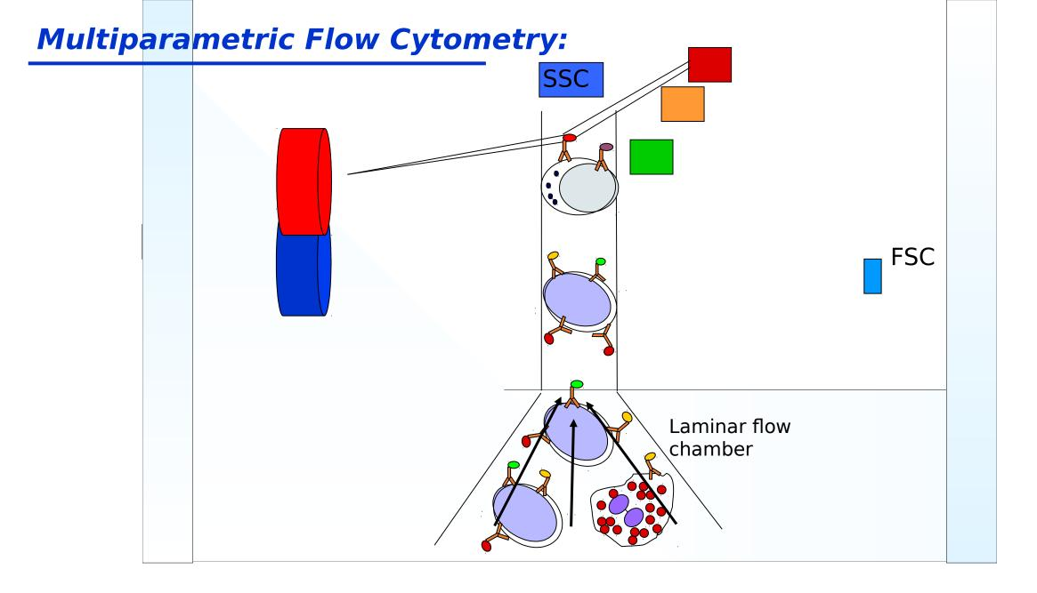
Flow Cytometers are able to perform fast evaluation of multiple parameters in millions of cells.
